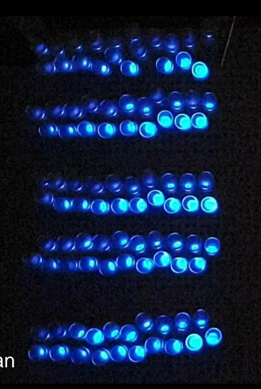
The 'cellulectric' TENG energizes up to **100 blue LEDs**, and as proof of concept and it can also be used to store electric charges in supercapacitors and small capacitors banks.
