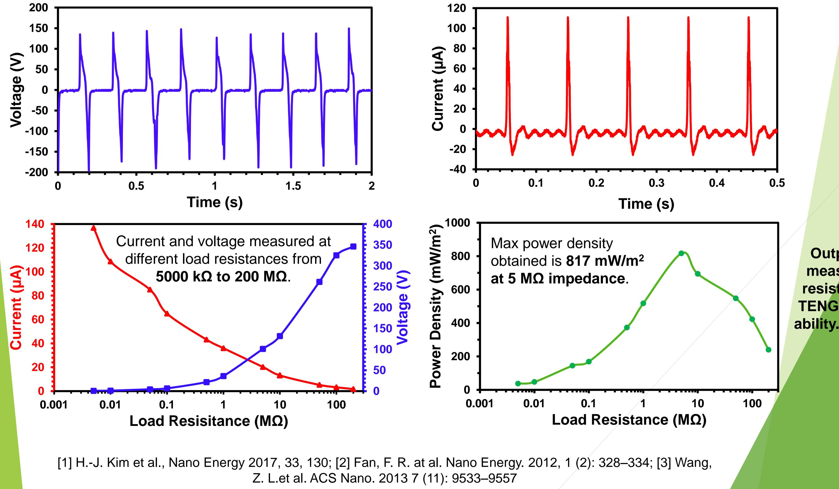
Absolute maximum current (Short Circuit Current,  $I_{SC}$ ) that the cellulectric TENG generates is **137 µA p-p**.
